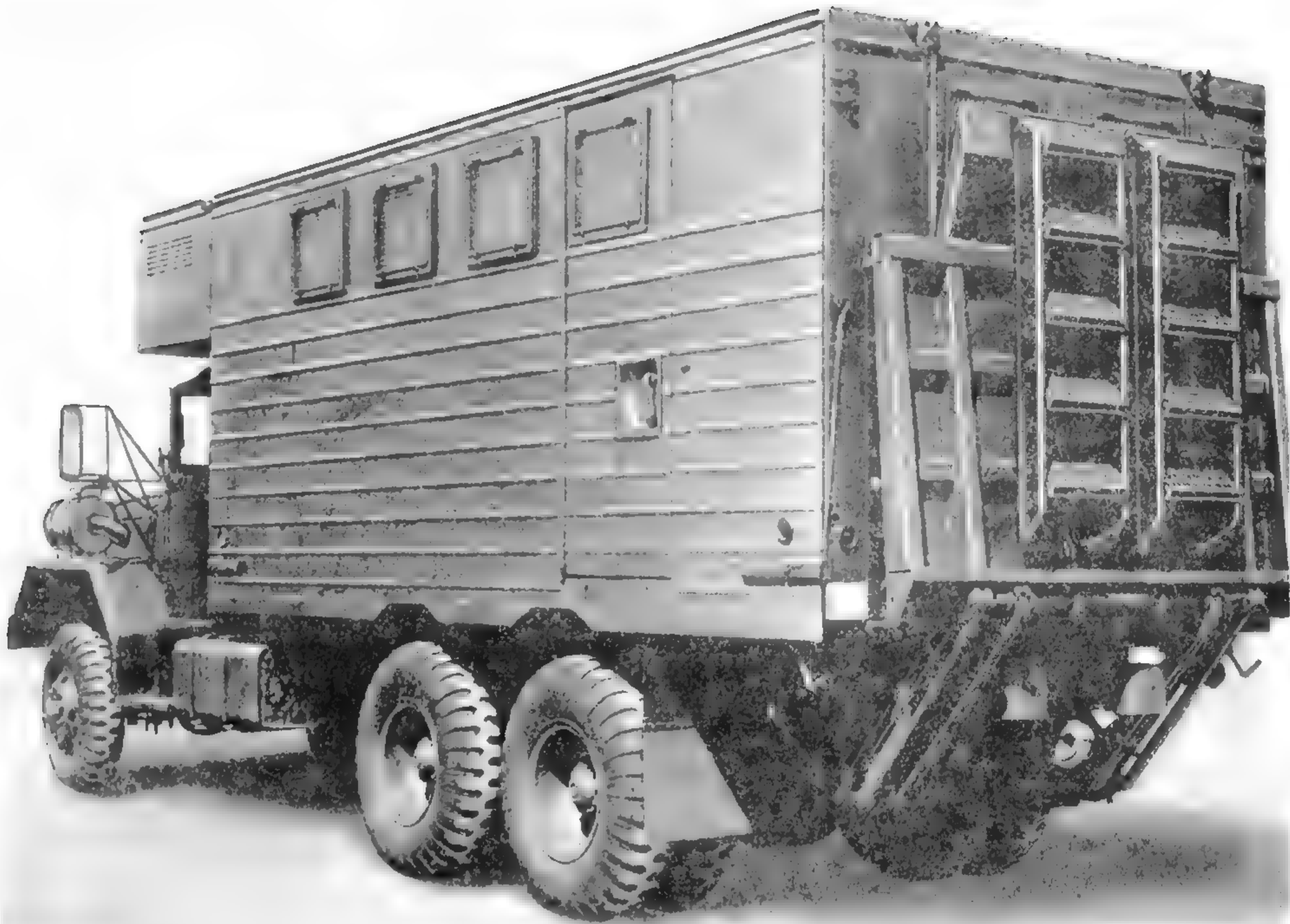
The power tailgate on the rear of the M820A2 could be powered by PTO, or electrically. This was very handy when moving large pieces of delicate electronic equipment. (U.S. Army photo)
